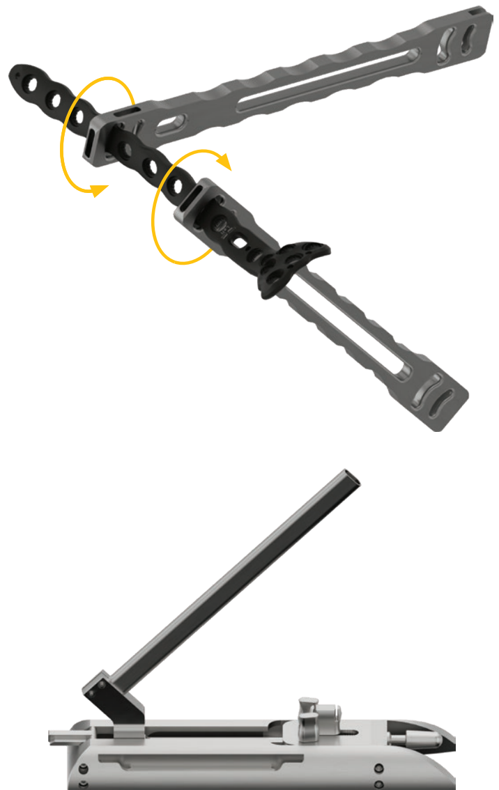
Fig 2. Bending Irons and Table Plate Bender
