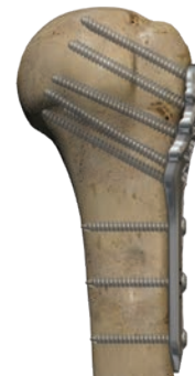
9. For additional shaft screws, use the 2.5 drill in neutral position
