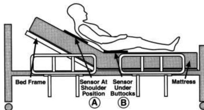
Figure 1 – Reprocessed Posey® Bed Alarm Sensor Pad Positioning
