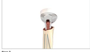
**Step 2**Prior to inserting final implant, drill in diaphysis to place two vertical tension NiceLoop sutures as demonstrated above.
