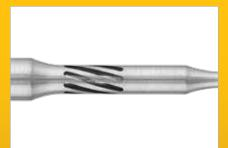
Helical reliefs redirect the ultrasonic energy from purely longitudinal to combined torsional component so tissue distal to the tip is unaffected by cavitation.
