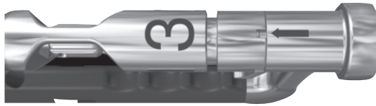
FIGURE 37 Alignment of Position 3.
