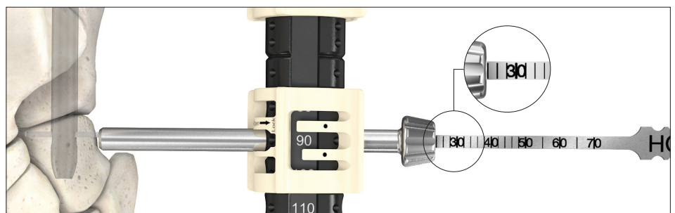
Screw measurement using depth gauge
