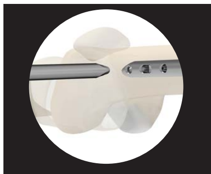
Fig. 115: Sleeve and nail tip are parallel and collinear. No adjustments needed.
