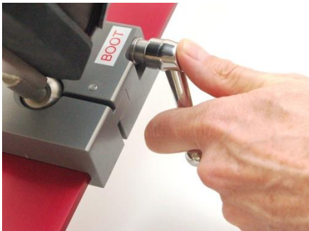
Fig. 3-39: Correct grip of the clamping lever
