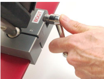
Fig. 3-4: Correct grip of the clamping lever
