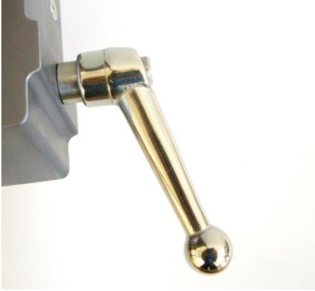
Fig. 3-8: Clamping lever turned downwards
