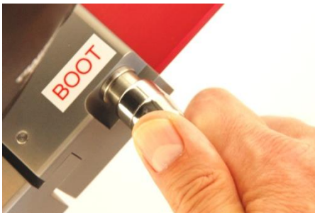
Fig. 3-6: Correct grip of the clamping lever
