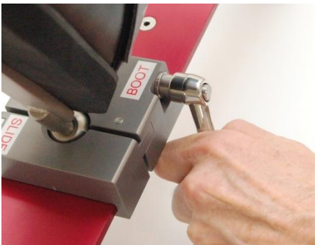
Fig. 3-3: Incorrect grip of the clamping lever
