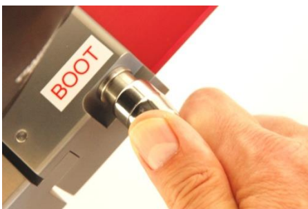
Fig. 3-41: Correct grip of the clamping lever
