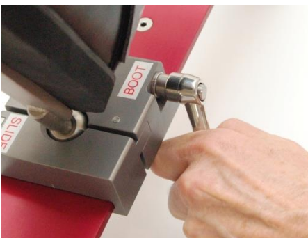
Fig. 3-38: Incorrect grip of the clamping lever
