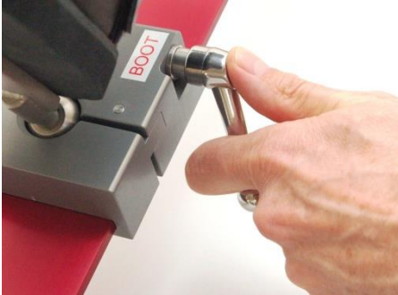
Fig. 3-28: Correct grip of the clamping lever
