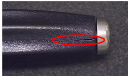
Cracked handle grip
