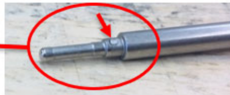
Femoral Array Post Pin Failure
