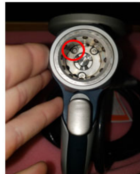
MICS Handpiece Locking Mechanism Screw Shear
