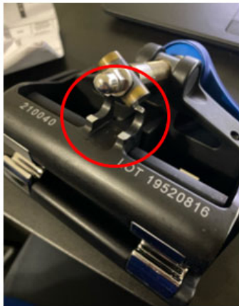
Rail Clamp Housing Fracture
