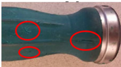
Damaged silicon handle
