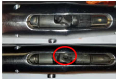
Offset Reamer U-Joint Deformation
