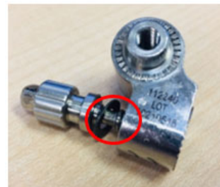
Pelvic Array Adapter, Internal Pin deformation allowing screw dissociation
