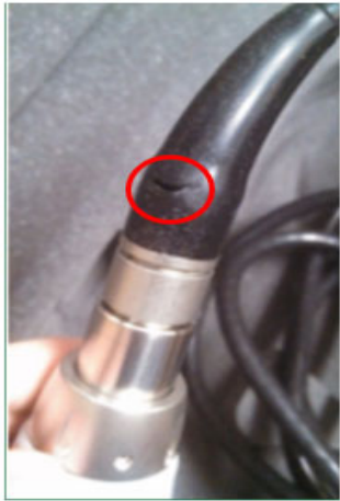
MICS Handpiece Cable damage
