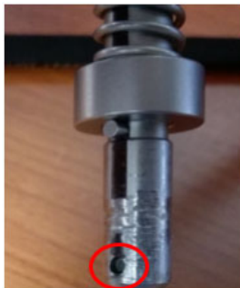
Base Array Connection Post, Pin Fracture
