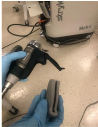
MICS Handpiece Handle Screw Missing causing handle dissociation
