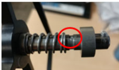
Base Array Connection Post, Pin Fracture
