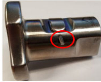
Impaction Platform Pin Protrusion
