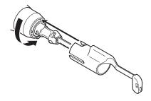
Release the guard collar lever. Make sure the guard collar returns to its original position and the blade guard is securely locked in the guard collar.
