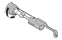
Release the guard collar lever. Make sure the guard collar returns to its original position and the blade guard is securely locked in the guard collar.
