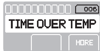
Figure 13 – Total Time Exposed to Over Temperature Conditions
