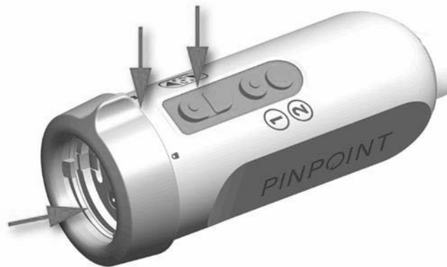
Figure 56: Hard to reach areas on the PINPOINT camera
